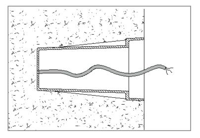
GB: Recess the protection cage into the concrete, taking care this is correctly aligned with the surface level.
