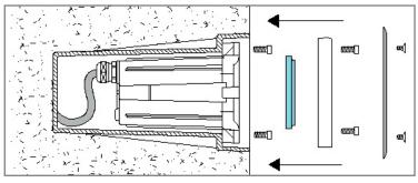
GB: Screw the housing to the sleeve, lay the diffuser, overlap the aluminium ring and screw tightly.
