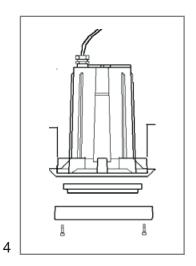
Place the aluminium ring in position and block using the screws supplied. (max. 2N/m)
