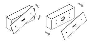
Make two hole for fix the bracket with a distance of 120mm
